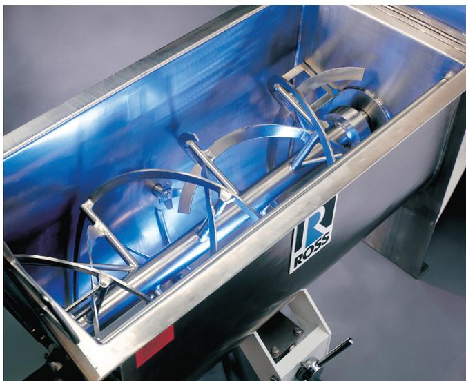
**Anatomy of a ribbon blender:** The inner and outer ribbons in this Charles Ross & Son Co. ribbon blender are pitched to move material axially, in opposing directions, and also radially. This combination promotes high-speed diffusion, convection, and shear.
