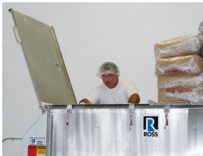
**Small details in design and finish—such as radiused corners and a highly polished trough—accelerate the ribbon blender’s changeover between batches. Total Nutrition Technology cut changeover from 25 minutes to 10 and significantly improved throughput.**
