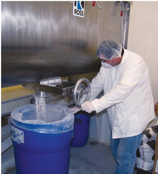
**The electronic variable-speed control of the Ross ribbon blender, combined with a precise gear-driven valve, enables fast and accurate discharge of solids over a broad range of densities and flow characteristics.**
