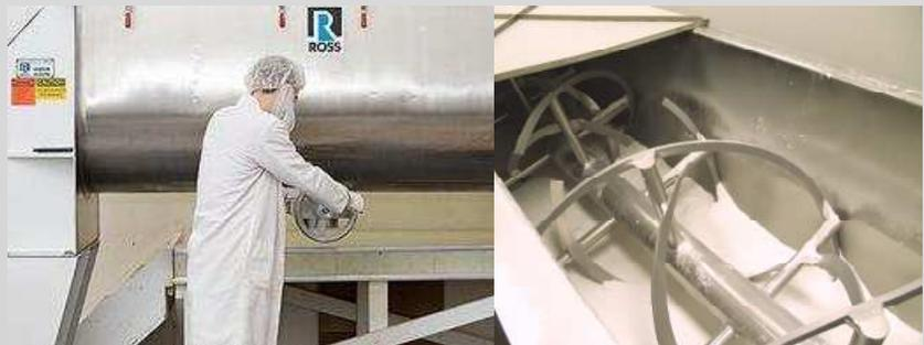
Shown is a Ross Ribbon Blender used for batching vitamin supplements and nutraceutical blends. In operation, ingredients are loaded into the blender, typically filling 40-100% of the rated capacity. This is up to the level of the outer ribbon's tip, leaving enough head space for the material to be vigorously agitated and mixed. Above photos show a batch during the discharge cycle.
