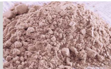
The thermoplastic resin was previously being dried in a V-cone tumble blender and transferred to trays for curing in an oven. Afterwards, the powders are milled to disperse agglomerates that have re-formed during curing. This three-step process took 24 hours to complete.
